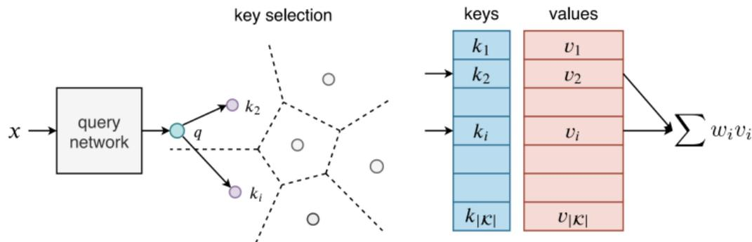
Figure:  $x$ , the input, processed through the query network, produces a query vector  $q$ , which is compared to all the  $|\mathcal{K}|$  keys, and then output the **sparse** weighted sum of over the memories associated with the selected keys. All parameters of the memory are trainable, while only  $k$  selected memory slots are updated for each input.
