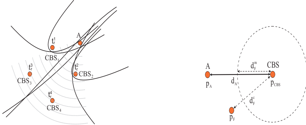
Figure 7: Infrastructure-centric and Node-centric Positioning based on covert base stations[CCS06]
