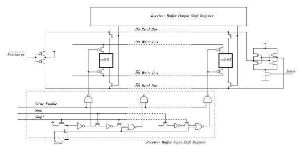
Fig. 4: FIFO Buffer Design
