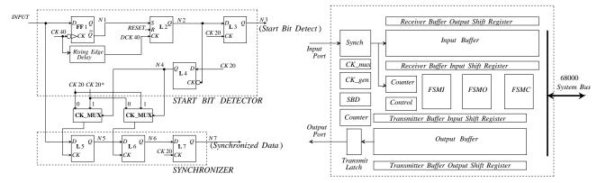
Fig. 1: Input Port Synchronizer
