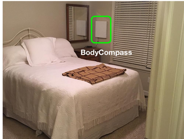
Figure 7-1: BodyCompass in one of our deployments. The white box mounted on the wall is the radio. It uploads the RF signals to the cloud where the model processes them to extract sleep posture.
